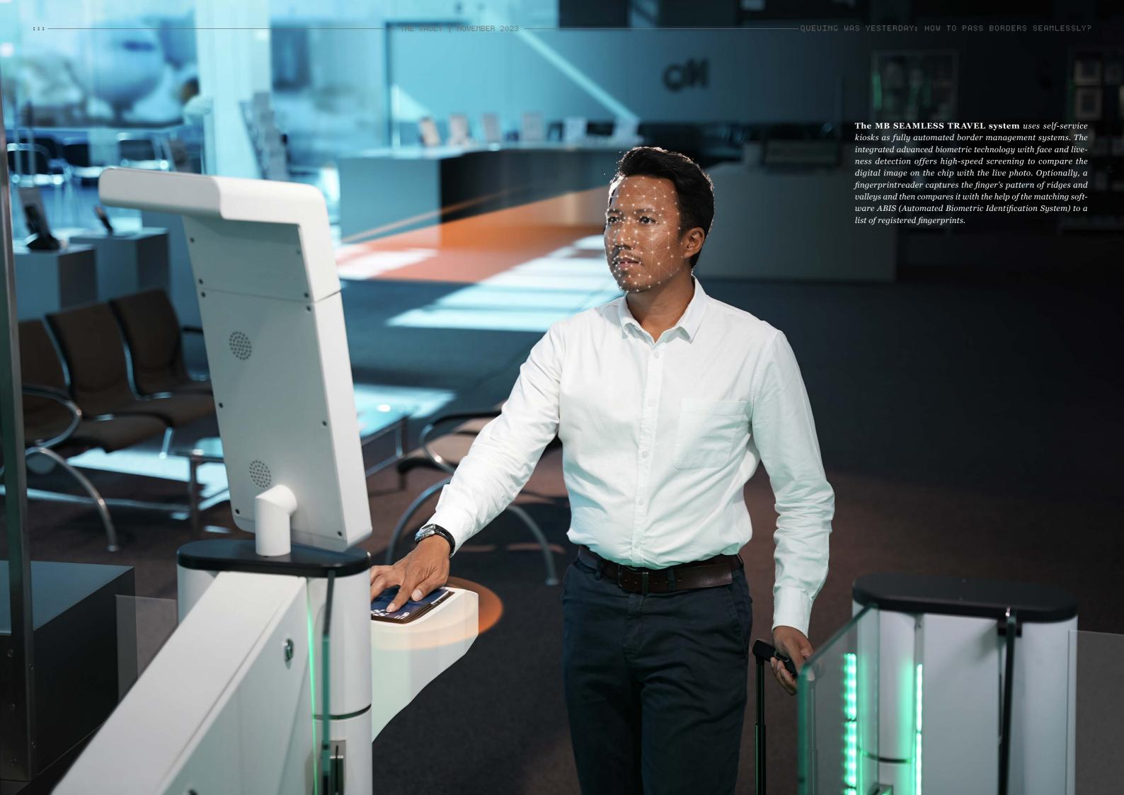
reader captures the finger's pattern of ridges and valleys and then compares it with the help of the matching software ABIS (Automated Biometric Identification System) to a list of registered fingerprints. Besides the whole verification tools, the MB iKiosks can be equipped with a barcode reader and a thermal printer to scan or print the flight tickets. Although it sounds like a long process with many individual security steps, the complete registration only takes around 15 seconds.
