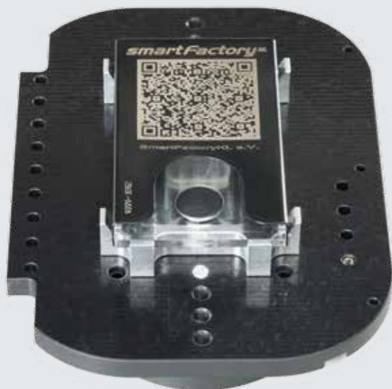
↑ Individual laser engraving on the top side
