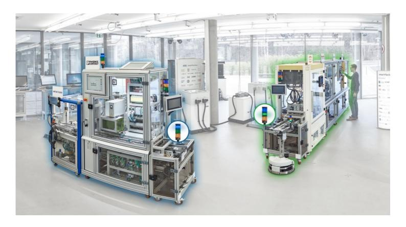
The Industrie 4.0 demo production plant of the *SmartFactory*<sup>KL</sup> consortium uses a dynamic safety concept. The result: The ability to parameterize individual production cells in emergency stops.
